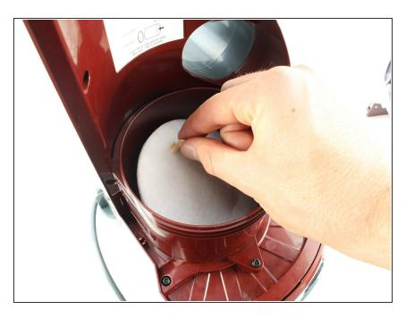
Pull up on the small tab to remove the filter pad.
