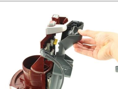
Use the metal spudger to pry off the back panel.
