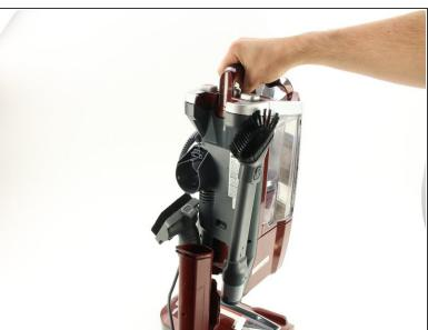
Press the Lift Away button and pull up on the handle to separate the top of the vacuum from the bottom.
