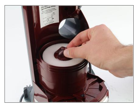
Pull up on the filter tab to remove the large foam filter.
