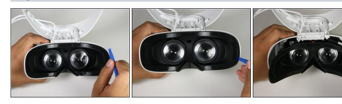
• Remove the cover using one of the plastic opening tools, and then carefully pull it from the casing.
