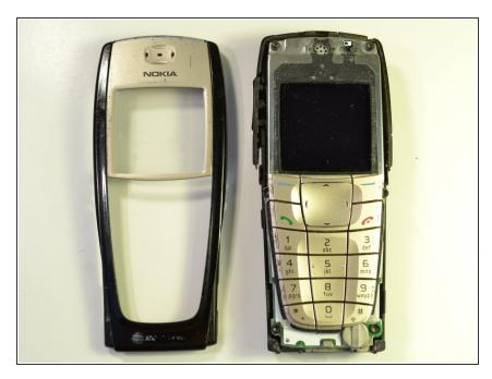
• The keypad and LCD screen are revealed.
