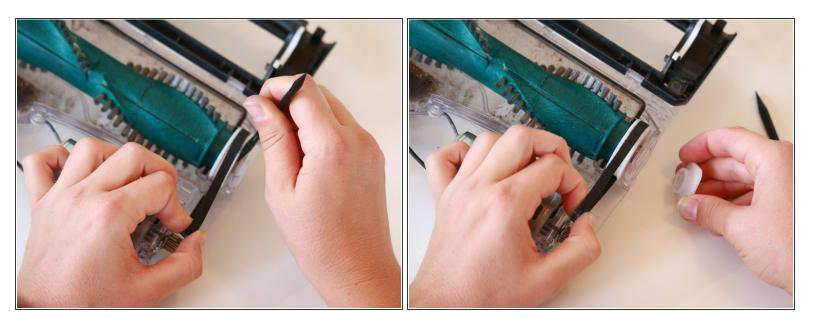
Using the spudger, push the white end cap out of the clear plastic by placing the spudger on the roller brush side and pushing the cap outward.
