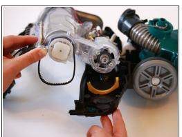
Remove the visible side of the belt from the gear with a spudger.
