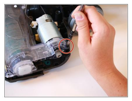
Remove the single 13.4 mm screw located next to where the belt was detached, securing the motor in place, with a PH1 screwdriver.
