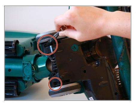
Remove the two 15.9 mm screws from behind the wheels with a T20 bit screwdriver.
