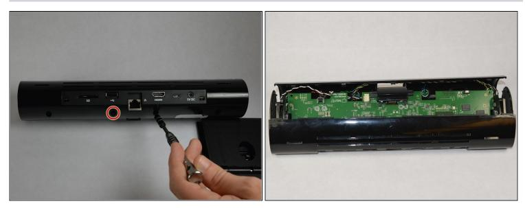
• Remove the 1.2 cm hex T9 screws and gently open up the device.
