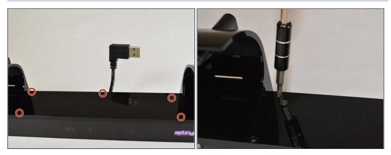
• Flip the top bar over and using a #00 phillips head screwdriver, remove the five 7mm screws holding the bar together.
