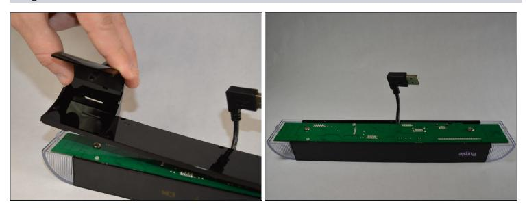
• Carefully pry off the plastic panel, revealing the motherboard.
