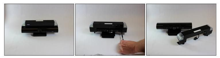
• Remove the top bar by removing the 5cm hex T10 screws on the back of the device as shown. Then gently pull off the top bar from the main component.
