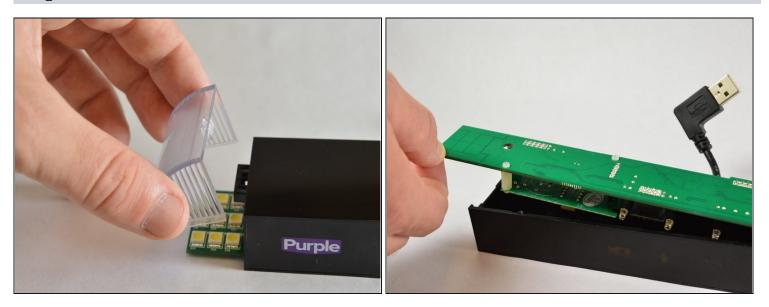
• To release the motherboard from its plastic housing, first pull the plastic light covers up and away from the device.
