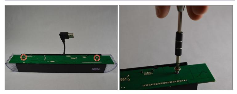
• Remove the two 7mm screws holding the motherboard in place with a phillips head screwdriver size #00.
