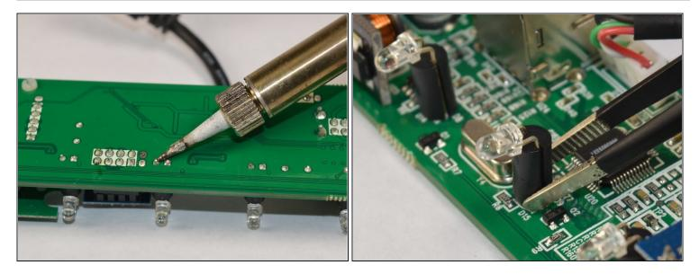
• Heat the solder on the underside of the affected light to remove and replace it using <u>tweezers</u>.
