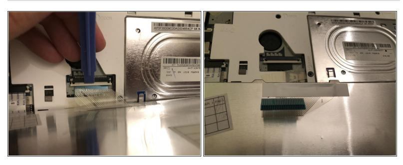
Unclip and disconnect the connector to remove the keyboard
