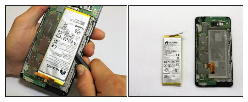
• Use the spudger to pry the lithium battery away from battery compartment.
