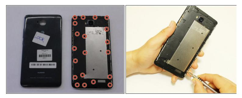
• Use a Phillips screwdriver to remove 20 screws around the perimeter of the phone.
