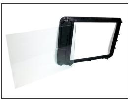
Remove the glass pane by carefully bending the plastic frame down from the side and sliding the glass pane out from the side.
