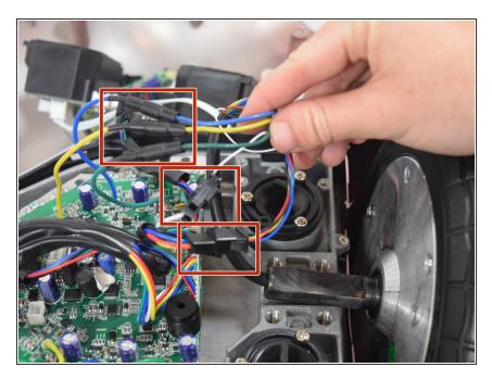
Check that all the clips are secured properly.
