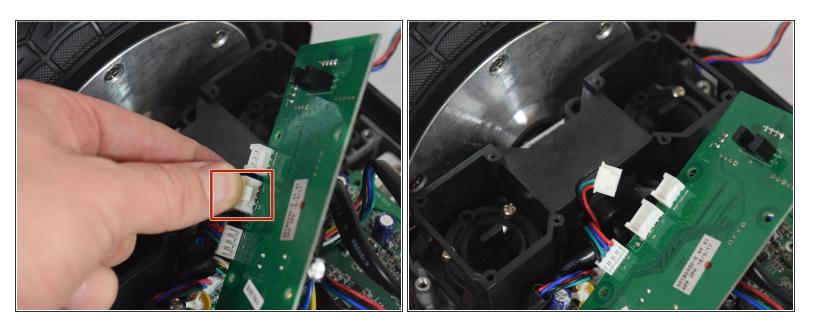
Remove the middle connector by squeezing the top of the tab and pulling up.
