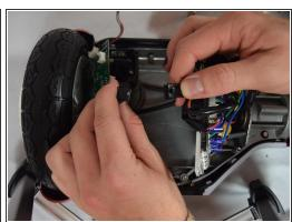
Unclip the black connector by squeezing both sides and pulling them apart.
