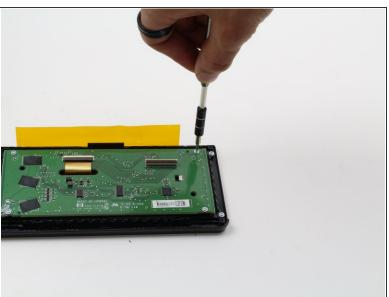
Remove the four 4.8 mm T6 screws from the back of the display motherboard.
