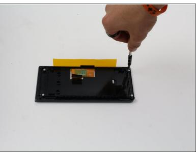
Remove the four 4.8 mm screws from the back of the display using a T6 screwdriver.
