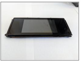
Lift the display out of the case.
