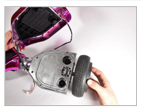
Turn the board over and pull the top panel off.
