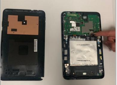
Disconnect the battery from the motherboard by pulling the side of the black plastic up.
