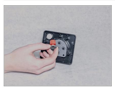
Remove the button from the joystick housing. Check for dirt or debris that may obstruct its movement. If the button is broken, replace it.
