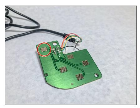
Inspect the circuit board for dirt, corrosion or damage. If necessary, clean the indicated contact using a cotton swab.
