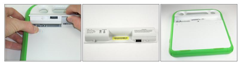
• Lift the middle of the battery to remove it.
