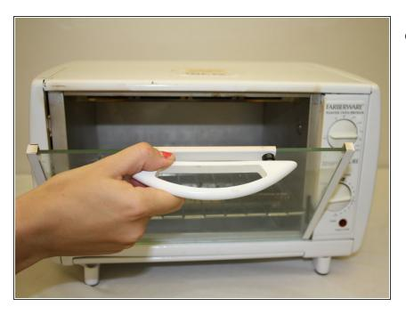
Hold firmly for a minute to allow glue to properly set.
