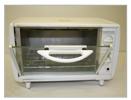
Replace the handle in its original position on the door.
