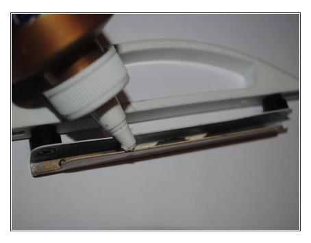
Apply glue to the inside of the bracket on the handle.
