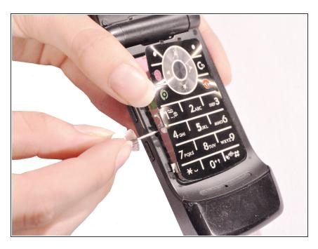
Insert a push pin into the notch located on the left side of the keypad and push the pin under the keypad membrane.
