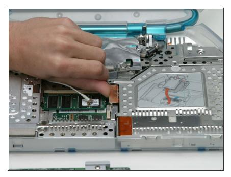
Disconnect the optical drive cable from the logic board.
