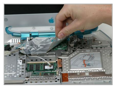
Peel the modem shield away from the metal framework below, working from the right front and moving to the left.
