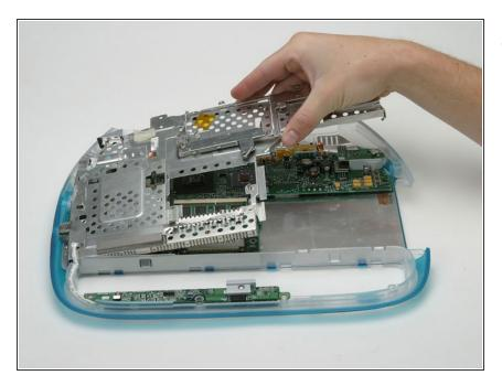
Lift the right side of the EMI shield up and pull it out of the computer.
