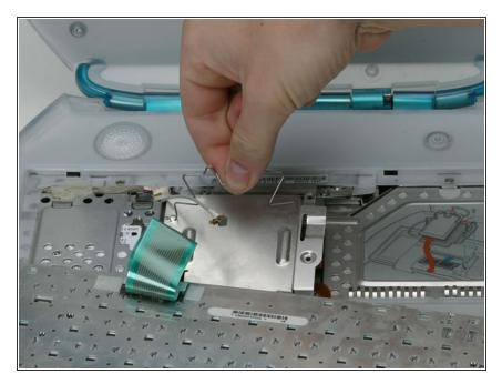
Grasp the wire metal bracket on top of the RAM shield and pull upward to remove the shield.
