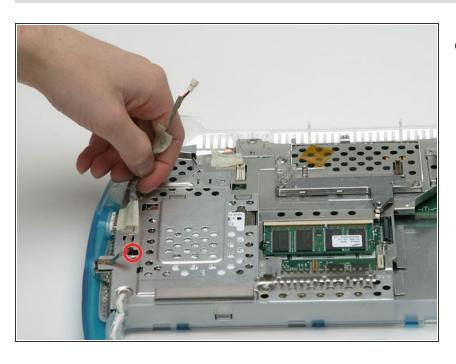
Deroute the speaker cable from the metal framework and disconnect it from the logic board.
