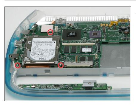
Remove the three 5 mm standoffs securing the hard drive to the logic board.
