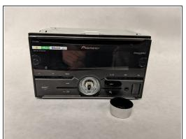
Remove the volume knob by pulling it away from the face of the radio receiver.
