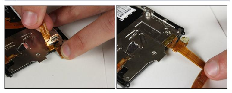
$\triangle$  Carefully pull the long orange cable away from the device.
