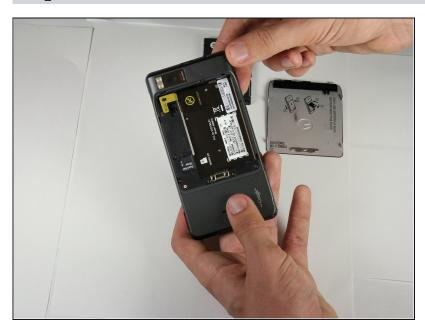
The battery has been successfully removed.
