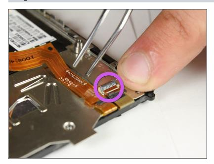
Flip up the cable connector and pull out the small flat cable.
