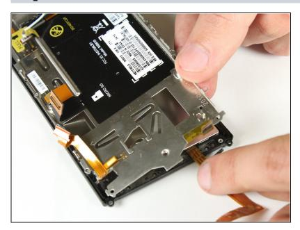
Carefully separate the metal plate from the LCD and front housing.
