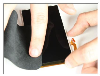
A Remove all dust and smudges from the LCD and front housing before installing the screen.
