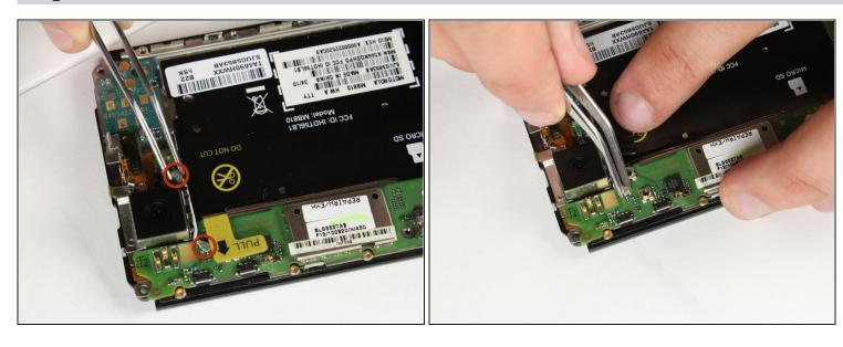
• Carefully remove the white connecting wire from the motherboard using <u>tweezers</u>.
