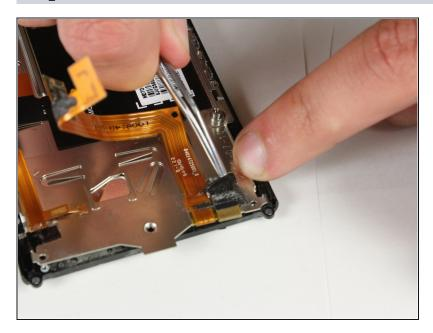
Peel black the black electrical tape located near the bottom of the device.
