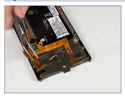
Using tweezers, peel the orange and black cable away from the device, stopping before reaching the electrical tape at the near the edge of the screen.
