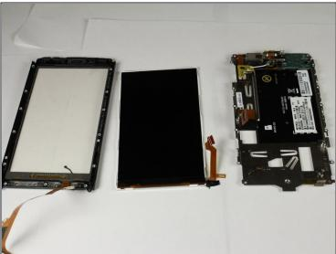
• Lift the LCD out of the front housing.
