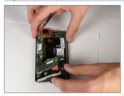
Carefully lift the motherboard and camera module up. Do not remove it from the phone!
