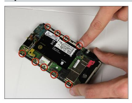
Remove the screws along both sides of the motherboard using a T3 Torx screwdriver. On some phones this may require a #1 Phillips Screw Driver.
