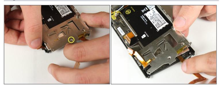
ullet Unscrew the screw at the base of the screen using the T4 torx screwdriver .
