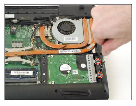
Remove the two 5 mm black screws on the right hand side with a Phillips #0 screwdriver.
