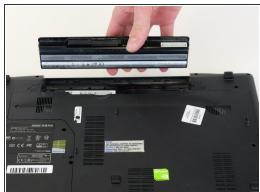
While holding the release tab, remove the battery slowly.
