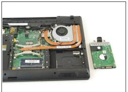
Lift the hard drive, then remove from the device. There is a black strip of plastic attached to make the process easier.
