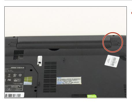
Find the unlock tab located on the upper right side of the device, then slide it to the right.
