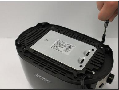
Use a Phillips #2 screwdriver to remove all of the 6mm screws from the bottom of the toaster.
