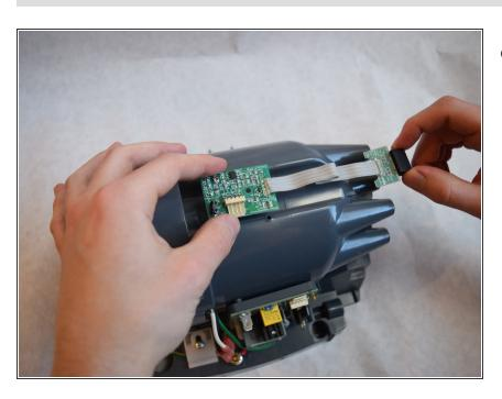
Carefully remove the sensor board from your device.
