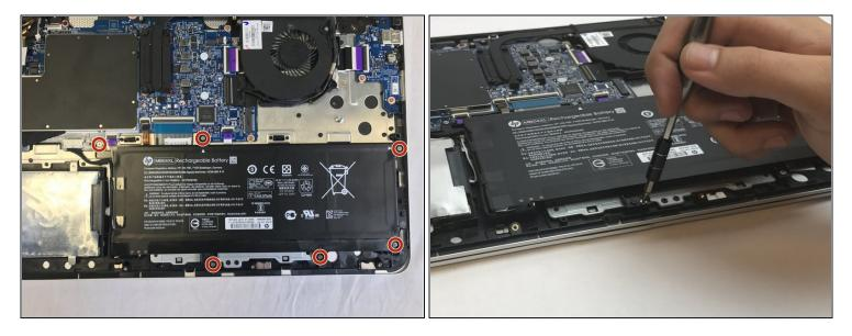
• Use a JIS #1 screwdriver to remove the six 4.7 mm screws.
