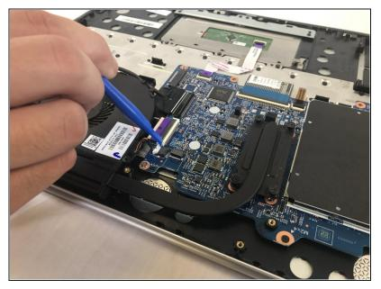
• Use the plastic opening tool to disconnect the power cable from the fan.
