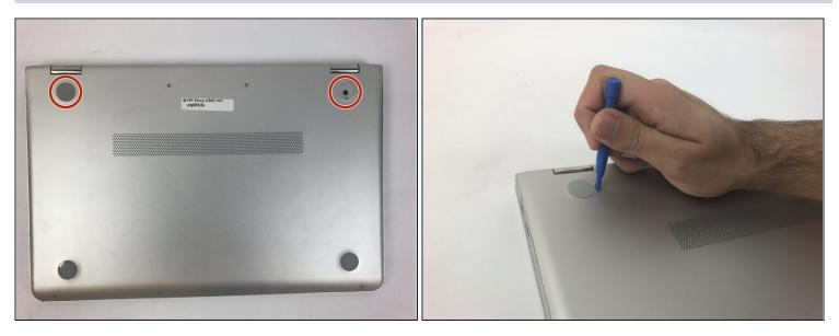
• Use the plastic opening tool to remove the gray rubber pads on the bottom of the laptop. For our device we only needed to remove the two at the top.
