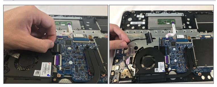
• Use your fingers to lightly pull the cable and disconnect it from the motherboard.
