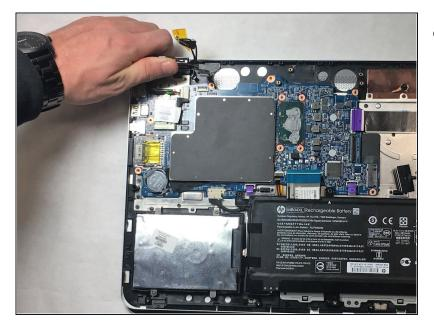
• Using your hand, lift the screen hinge located in the top left corner. This will allow for easier removal of the motherboard.
