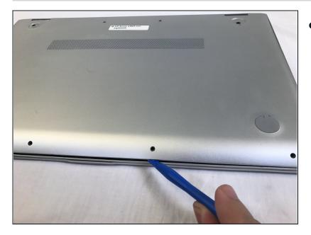
Use a plastic opening tool to pry open the case. Go slowly around the edge. You will hear popping noises, such are due to popping open the small joints that keep the cover attached.
