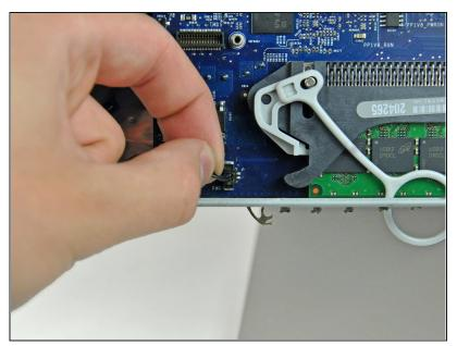
Disconnect the power button cable by pulling its connector away from the face of the logic board.
