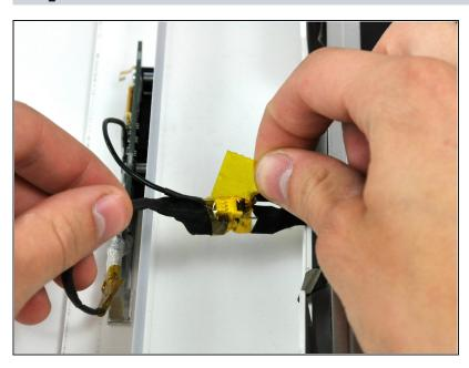
If necessary, remove the piece of kapton tape wrapped around the microphone and camera connectors.
