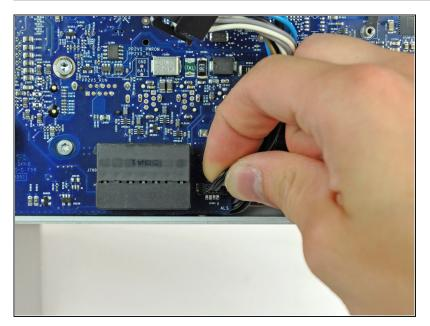
Disconnect the ambient light sensor by pulling its connector away from the face of the logic board.
