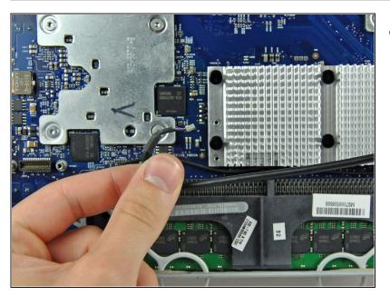
De-route the IR cable from under the aluminum heat sink and tuck it behind the optical drive to keep it out of the way.
