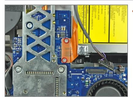
Remove the two T6 Torx screws securing the optical drive connector to the logic board.
