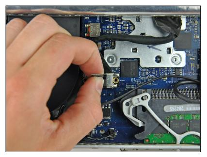
To disconnect the display data cable, grab its connector's black tab and pull it away from the face of the logic board.
