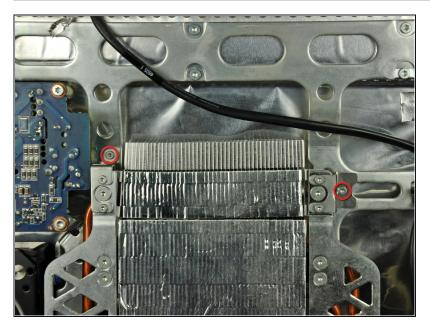
Remove the two T6 Torx screws near the top of the heat sinks.
