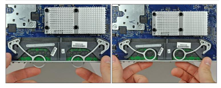
Tuck the RAM arms into the iMac so they rest on the perforated metal grille along its lower edge.
