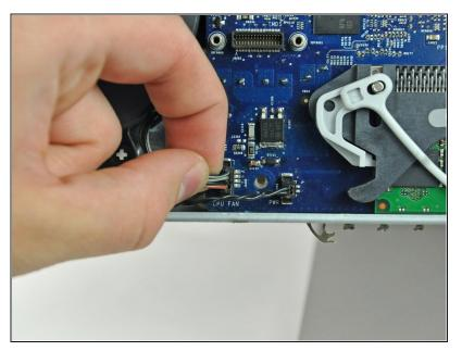
Disconnect the hard drive fan by pulling its connector away from the face of the logic board.
