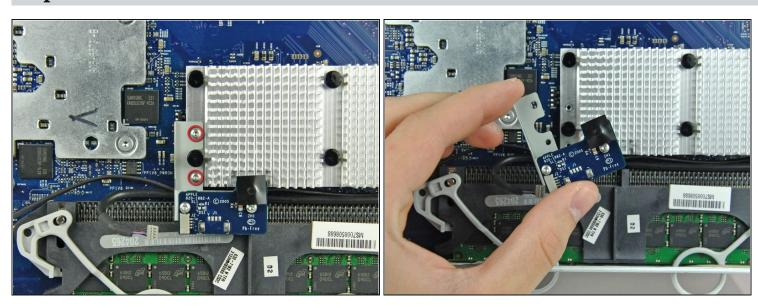
• Remove the two T6 Torx screws securing the IR board bracket to the IR board.
