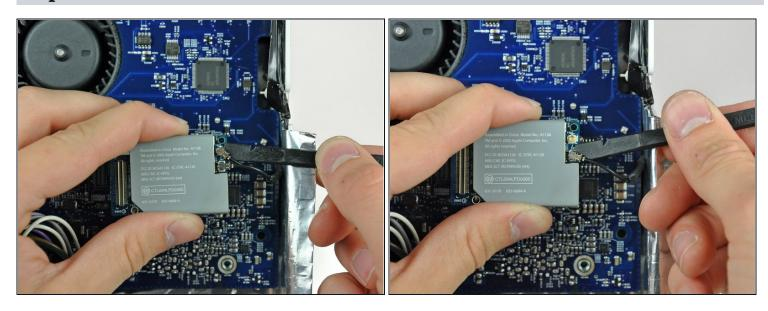
• Use the flat end of a spudger to pry both antenna cable connectors up off the AirPort/Bluetooth board.
