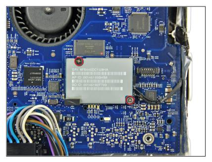
Remove the two Phillips or two T6 Torx screws securing the AirPort/Bluetooth board to the logic board.
