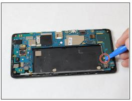
• Use a plastic opening tool to unplug the wires by pulling them to the side.
