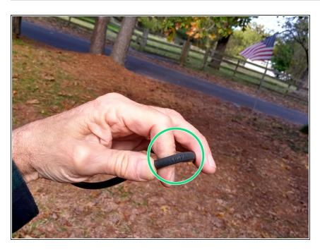
Bubbles visible in strainer chamber (or at outlet jets)? Bend oring at extreme angle as shown. If tiny fissures are apparent as in photo a new o-ring will solve the issue.
