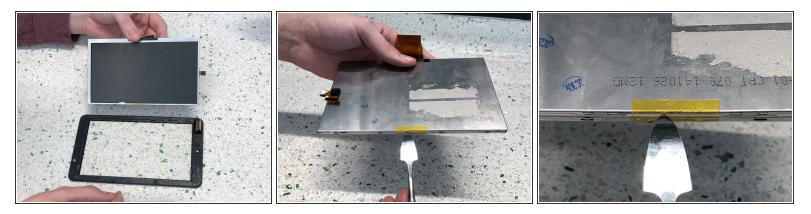
• Tear the yellow tape in order to make the front and back covers free to disassemble.
