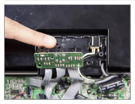
Pull out the AV circuit board and lift it up and out of the way to allow access to other components.
