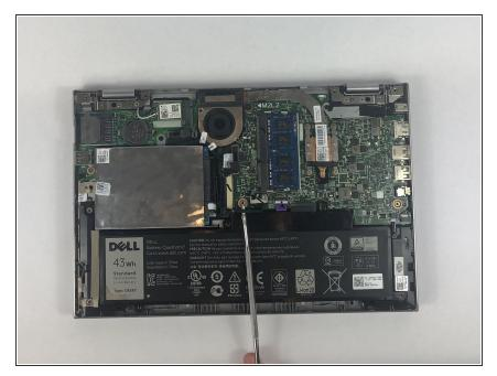
Remove the hard drive cable from the battery.
