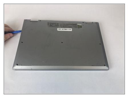
Use a plastic opening tool to remove the cover from the computer.
