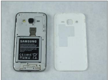
• Locate the battery near the bottom of the phone. The battery is square, flat, and is labeled 'SAMSUNG'.
