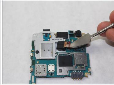
• Turn the Motherboard over and disconnect the ribbon connecting the camera to the Motherboard with an <u>iFixit Metal Spudger</u>.
