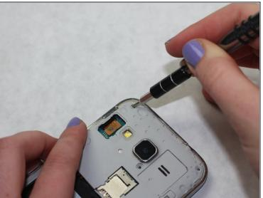
• Use a Phillips #00 screw driver to remove all eight 4mm screws from the midframe.
