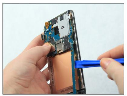
• Lift the motherboard from the phone with an <u>iFixit Opening</u> Tool.
