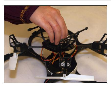
Carefully remove the drone body from the frame.
