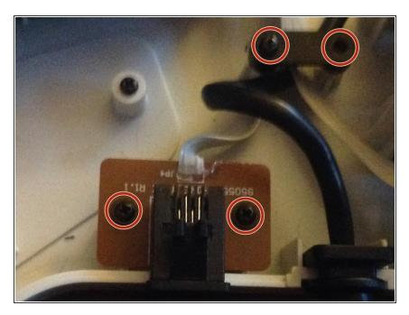
Unscrew the 4 Philips head screws.
