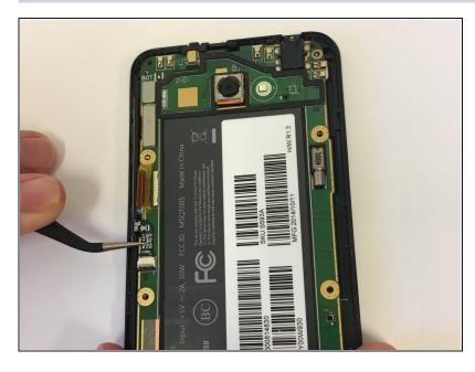
• Detach the black connector on the left hand side of the motherboard.
