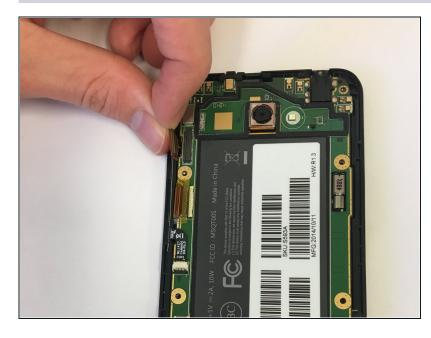
• Disconnect silver connector from the motherboard. It is located on the left hand side above the black connector.
