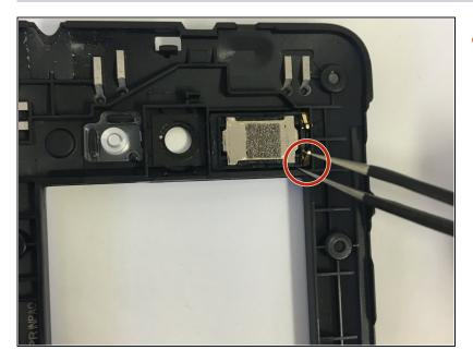
Remove speaker with standard <u>tweezers</u> to minimize damage, and replace.
