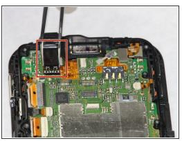
Remove final ribbon cable, lift the latch up, and then slide it down. The audio jack will then slide out.
