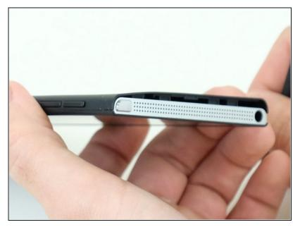
Gently pry up on the plate with the spudger. You may hear some cracking noises as you work the spudger around your device, this is normal.
