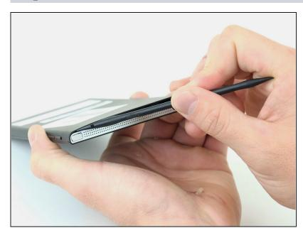
Obtain the black plastic spudger tool from the iFixit toolkit. Position the device as shown in the picture. Insert the flat end of the spudger directly in the space above the power button between the back cover and front screen.
