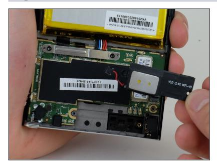
Remove the WIFI antennae from the device and replace.
