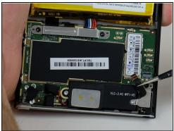
• Place the flat end of the black plastic spudger under the locking tab that holds the tail end of the black ribbon in place. Pry upwards unlocking the tail of the black ribbon. Use the tweezers to remove the black ribbon from the plug.
