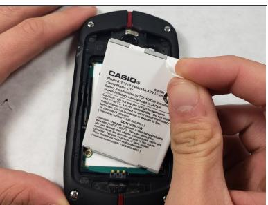
Pull the white battery tab upwards and remove the battery.
