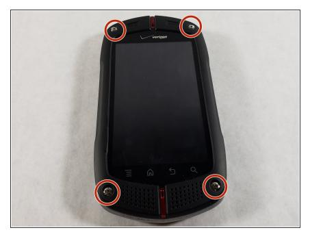
Remove the four 6mm Y0 screws from the corners of the device.
