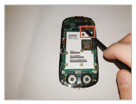
Using a spudger, pry away the motherboard from its compartment, by inserting the spudger in the compartment and lifting upwards until fully out.
