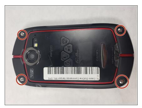
Remove the four 5mm Y0 screws from the back of the device.
