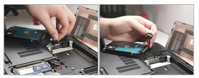
Place the old hard drive off to the side (as seen in photo) and carefully remove the SATA cable from laptop.
