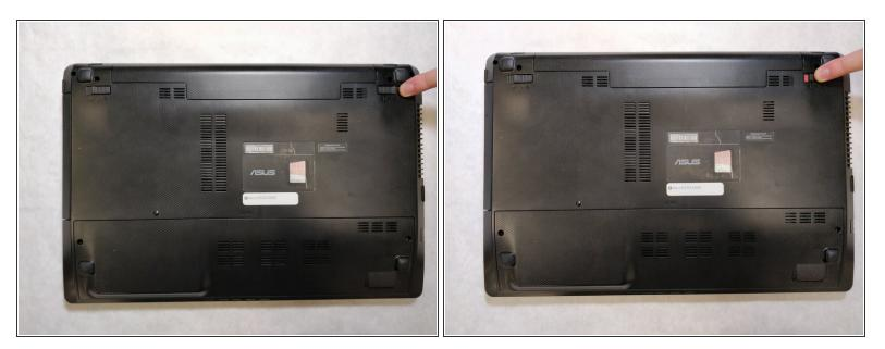
• Pull the latch to the right of the battery to the right.
