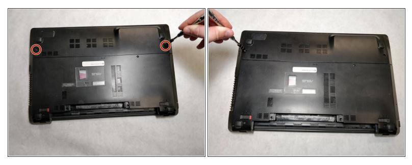
• Using a JIS #00 screwdriver, unscrew the two 5 mm screws on either side of the laptop panel.
