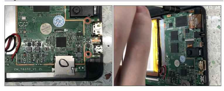
• Use a PH000 screwdriver to unscrew all four motherboard screws.
