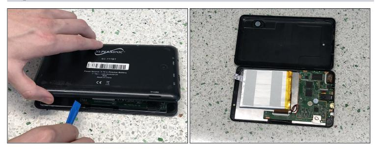
Pry open backing of the tablet using an iFixit opening tool.
