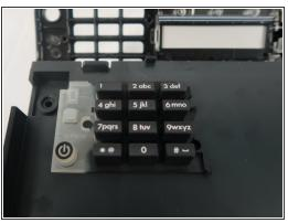
Remove the button that is located at the left of the controlling keyboard.
