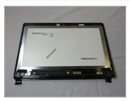
Remove the LCD Panel and faceplate from the device.
