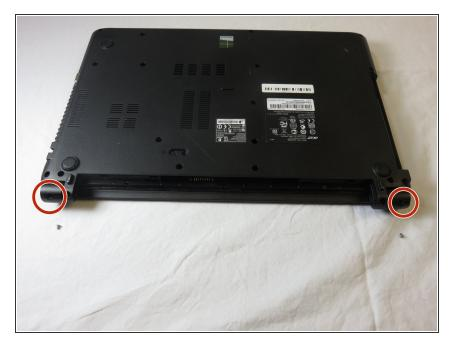
Locate the screws connected to the hinge of the laptop. Small, black stickers hide them from immediate view.
