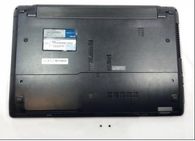
• Use the Phillips #0 screwdriver to remove the two screws circled in picture.
