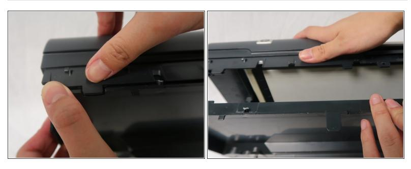
Using fingers to open the back cover board of the glass plate.
