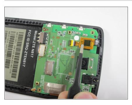
Use a pair of tweezers to gently disconnect the ribbon cable connector from its socket.
