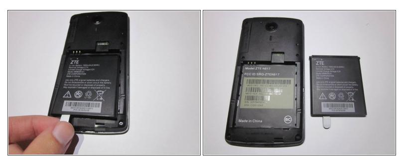
• Use the ribbon to remove the exposed battery.
