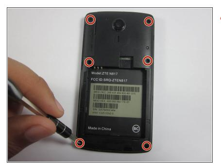
Use the JIS #000 screwdriver to remove the six 3.0mm screws placed in the back of the ZTE Quest.
