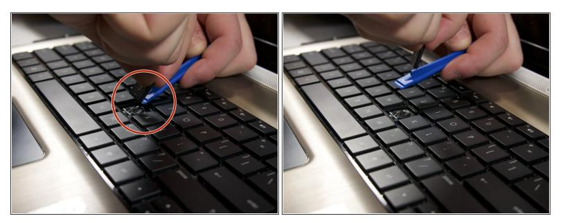
Remove the key by prying at the top part of the key using the plastic opening tool.
