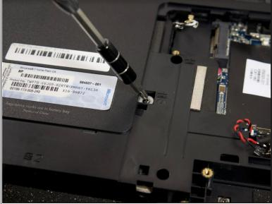
• Locate the screw that keeps the CD drive attached, and remove it with a Phillips head screwdriver.
