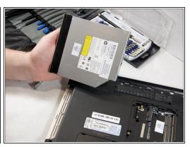
• After the screw is removed, pry the CD drive out of the laptop until you can grip and remove it.
