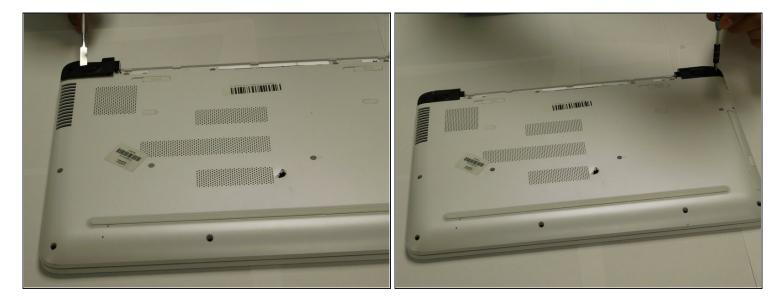
• Once the battery is removed, unscrew and remove the both of the 7.5 mm screws off the black tabs using a PH1 screw driver. Then pry off the covers using the plastic opening tools.
