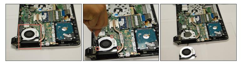
• Utilizing a PH00 Screwdriver remove the two 3.5 mm screws detaining the cooling fan. Then use tweezers to remove the plug connecting the cooling fan to the mother board. Lastly remove the cooling fan.
