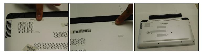
• Slide the tab marked with a lock/unlock symbol. The slide the other tab in order to release the battery.
