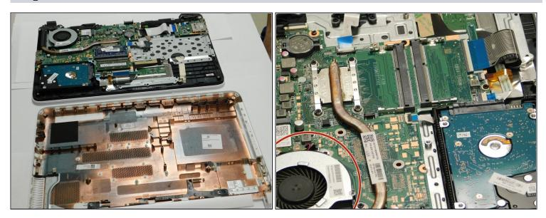
• Once the laptop is fully open locate the cooling fan.
