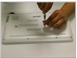
Locate all the screws and remove them with a 3.5 mm screw with a PH0 screw driver.
