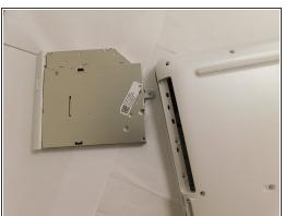
To pry the CD-Drive off the computer, just use a plastic opening tool. Then pull to remove the CD/DVD drive.
