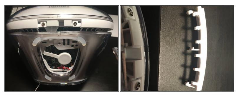
• Flipping the light upside down will present a small section of the bezel that can be pried upward. It is a small plastic strip with hooks that have to be disengaged to be removed.
